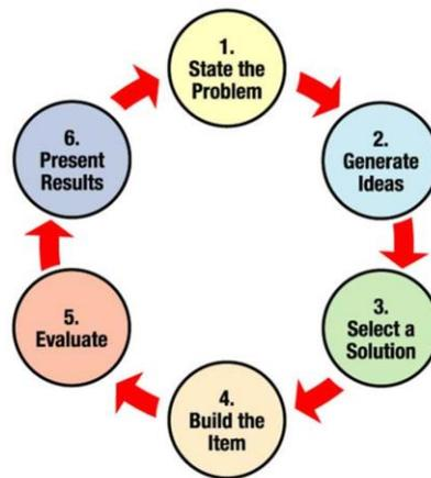
Figure 1. NASA Engineering Design Process (reproduced from (Rahman, 2014))
